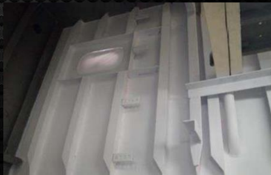
Insulation of interior surfaces on a patrol boat
